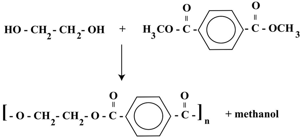
Figure 1.1: One route for the synthesis of PET.
